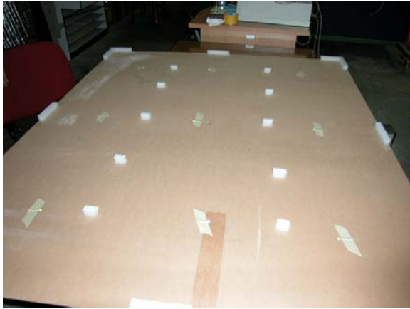
Figure 3 – Wood board with thermal probes placed inside.
